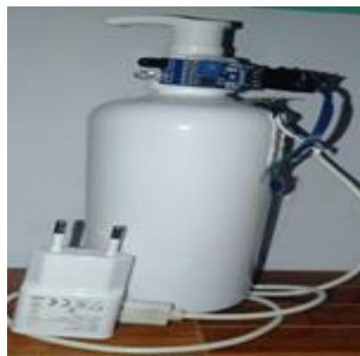
**Gambar 3.** Hasil Alat Hand Sanitizer Otomatis
